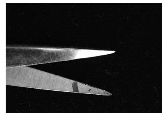
Pitting on a pair of plastic surgery scissors.
