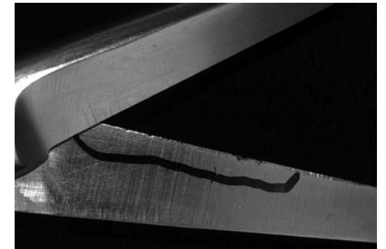
Staining and metal break-down on a pair of surgical scissors.
