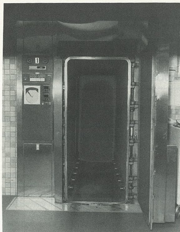
Photo of a steam sterilizer. The mechanical indicators on the left coincide with those illustrated on the previous page.
