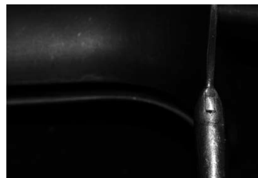
A flaw in a surgical vaginal speculum in which debris will accumulate.
