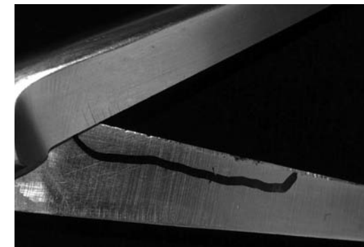
Staining and metal break-down on a pair of surgical scissors.
